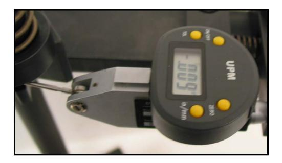
4. With the indicator point under the plunger face with the .009" to .012" reading on the indicator, press ZERO.
